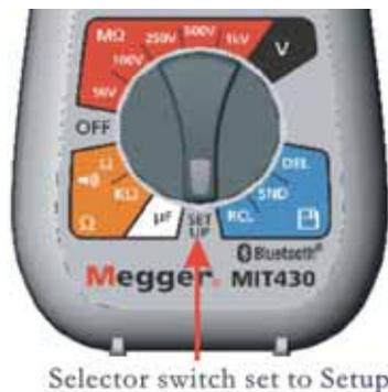
2. Scan for local “Bluetooth” computers. Press the yellow test button 5 times until the MIT430 / MIT485 displays “bt” with three dashes or a 3 digit number. (The three dashes indicate that the instrument has not yet been paired with a p.c., otherwise the current paired Bluetooth device ID will be displayed).
