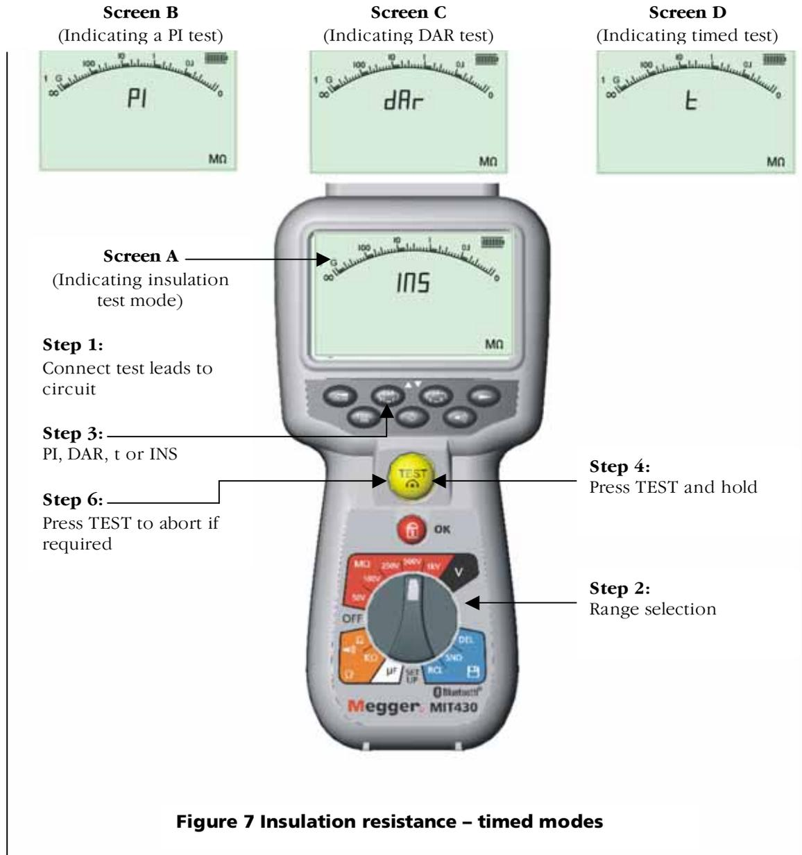
1. Connect the test probes to the isolated circuit under test.
