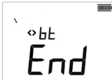
9. The MIT430 / MIT485 must now be switched to “OFF” after pairing to complete the process.
