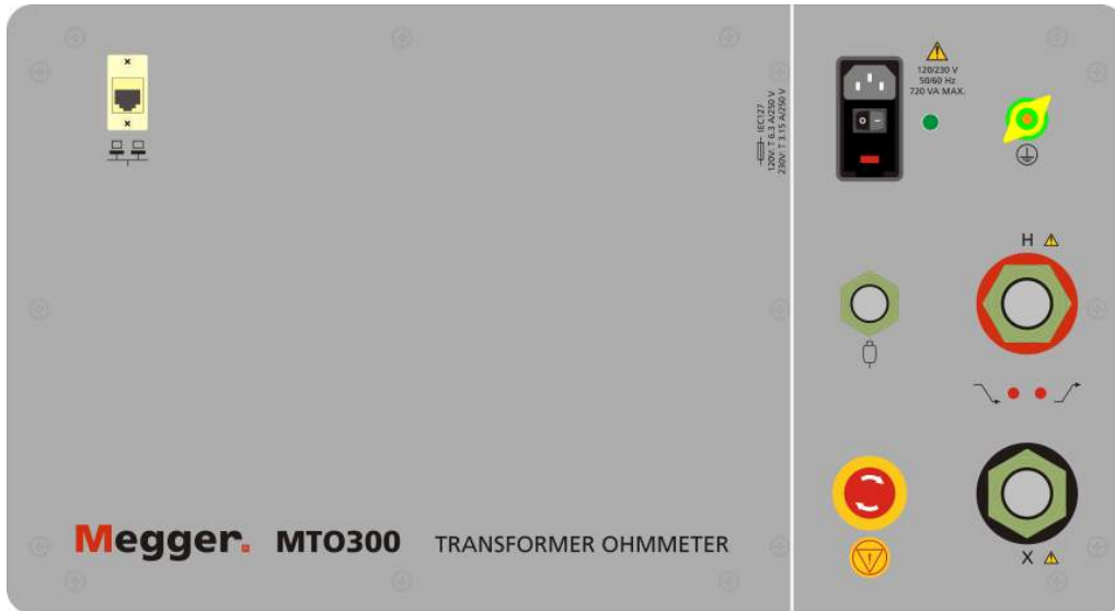
Figure 1: MTO300 Front Panel
