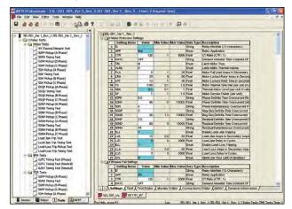
This example shows the organization tree descending by region, then substation, line, panel and finally the actual relay in the panel. The relays installed are then listed under that location. The heirarchial structure of AVTS includes up to 5 levels of organization.
