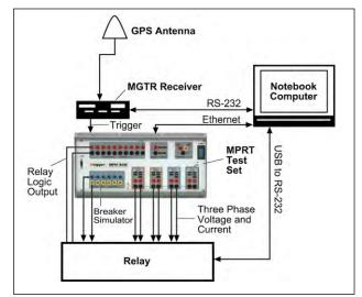
Typical End-to-End Test with MPRT
