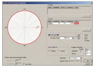
**Adjusting Ramp Control - Single Phase Current Increment**
