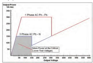
"PowerV" Voltage Amplifier Output Power Curves
