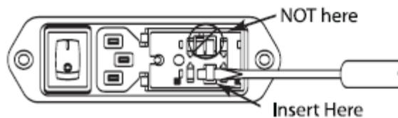
When the fuse holder is installed in the dual fuse position, it should normally release as soon as the door is open.
