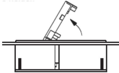
3. When the fuse holder is installed in the single fuse position, apply the screwdriver as shown and gently pry up. Use screwdriver as shown, do not use fingers.
