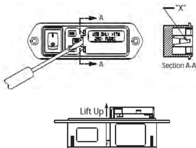
2. Once lifted, the door will pivot on its hinges and expose the fuse holder.
