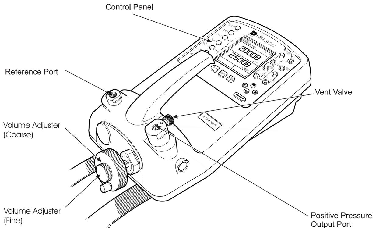
**Figure B1 - DPI 610LP Calibrator Controls**
