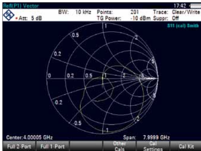
Vector network analysis: measurement with Smith chart.
