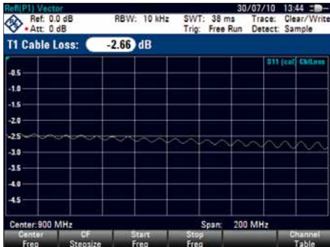
One-port cable loss measurement.
