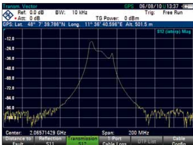
Display of current position during a transmission measurement with R&S®HA-Z240 GPS receiver connected.
