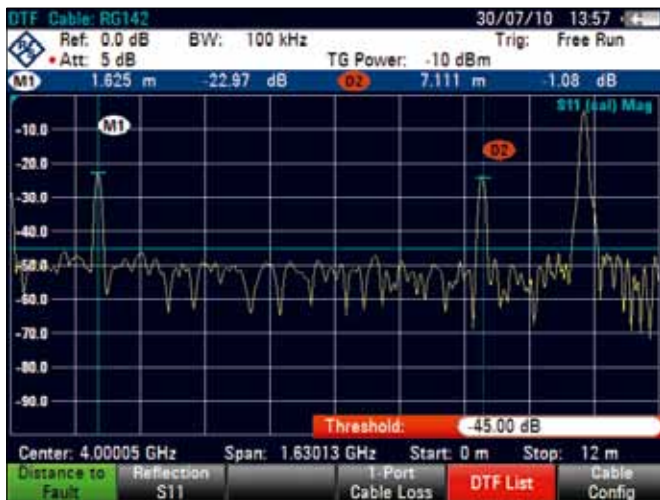
Distance-to-fault (DTF) measurement.
