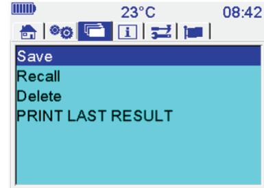
The user can select between internal memory and a USB memory device for the save, recall and delete functions. After selection of a memory location the relevant files are displayed on screen. Navigation is via the arrow keys as follows:
