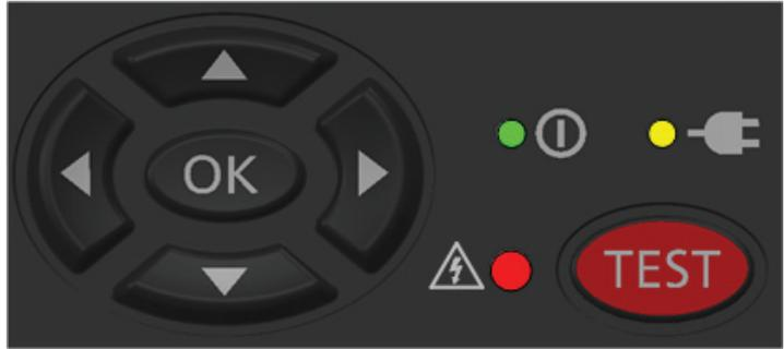
Within each user interface window the up and down arrow buttons are used to navigate up and down the functions listed on the left side of the screen. The 'OK' key either scrolls through options associated with each function or enters a lower level window to perform a function.
