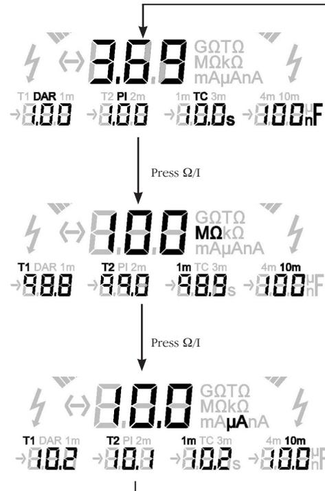
**Figure 3 - The result of a dielectric discharge test (DD)**
