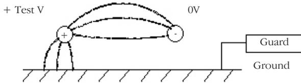
When making measurements above 100 G $\Omega$  therefore, the user should ground the Guard Lead where possible, otherwise parallel leakage paths may occur.
