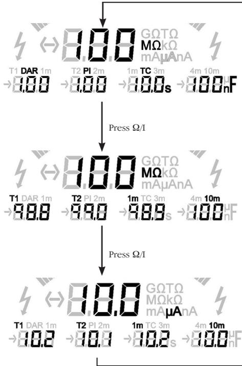
**Figure 2 - The result of a polarity index test (PI)**
