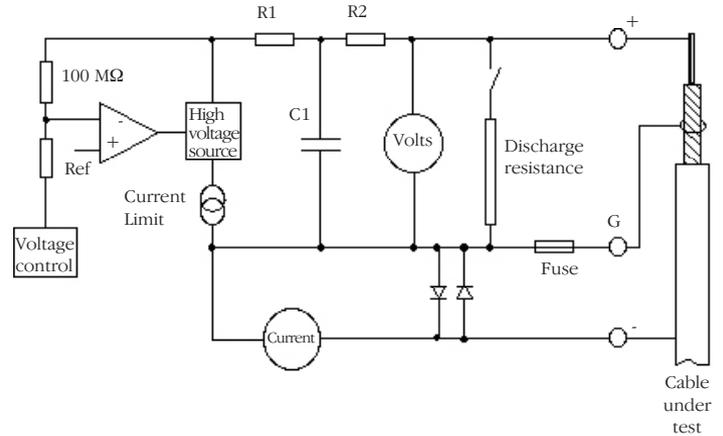
For 5 kV instruments  $C1 = 47 \text{ nF}$ ,  $R1 = 50 \text{ k}\Omega$ ,  $R2 = 40 \text{ k}\Omega$
