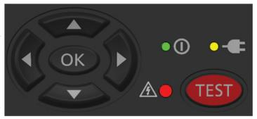
Left and right arrow buttons navigate between tabs on the top level window for optimum speed. Individual tab windows save the highlight function and return to the same position on each screen.
