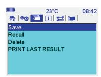
The user can select between internal memory and a USB memory device for the save, recall and delete functions. After selection of a memory location the relevant files are displayed on screen. Navigation is via the arrow keys as follows:
