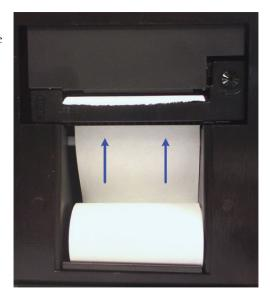
Holding the end of the paper roll, insert the paper under the cross bar and into the printer slot as shown (blue arrows) in the drawing opposite. Press the print feed key repeatedly until the paper is just visible feeding through the print mechanism.
