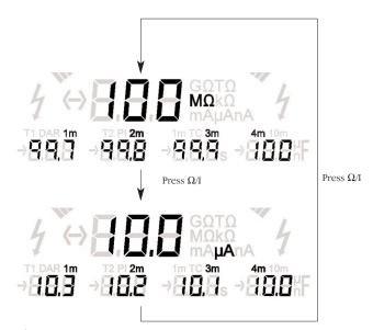
Figure 4 - The result of a step voltage (SV) test
