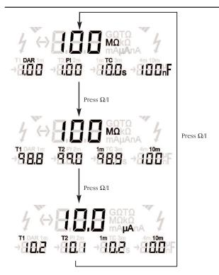
Figure 2 - The result of a polarity index test (PI)
