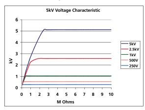
Test Voltage Output Characteristics Over Insulation Resistance Range 5-kV and 10-kV Insulation Resistance Testers
