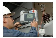
Circuit breaker being tested with the S1-552/2
