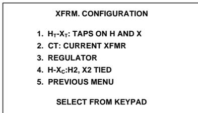
Figure 6-4a. Additional Single Phase Transformer Configuration Screen
