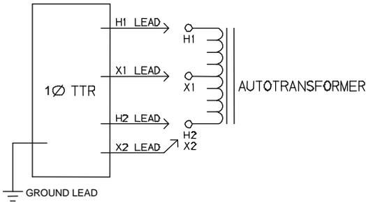
Figure 5-2. Setup for Testing Single-Phase Autotransformer
