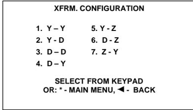
Figure 6-5. Three Phase Transformer Configuration Screen
