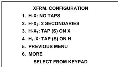
Figure 6-4. Single Phase Transformer Configuration Screen
