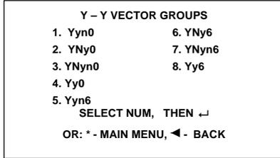
Figure 6-5a. Three Phase Transformer Configuration Screen
