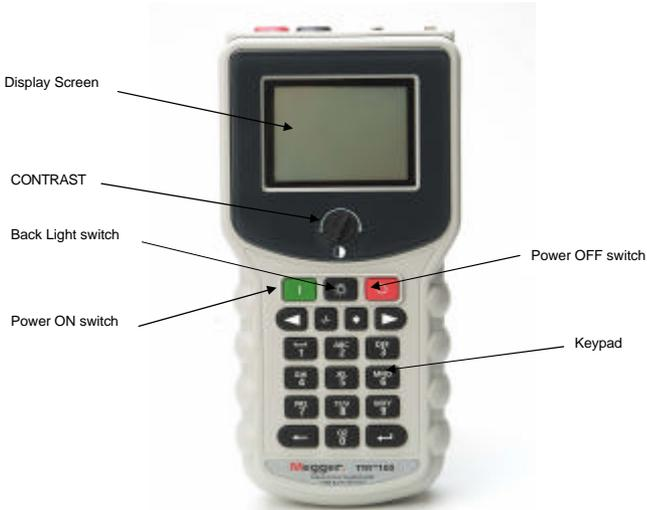
Figure 4-2 Single-Phase TTR Display & Control Panel
