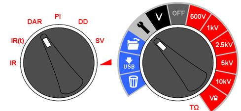
DAR and PI timers t1 and t2 are set when DAR or PI is selected on the test mode rotary switch with the central rotary switch in the settings position. Timer t1 is set first followed by t2. Up and down arrow buttons are used to change the t1 and t2 default values and OK confirms each setting.
