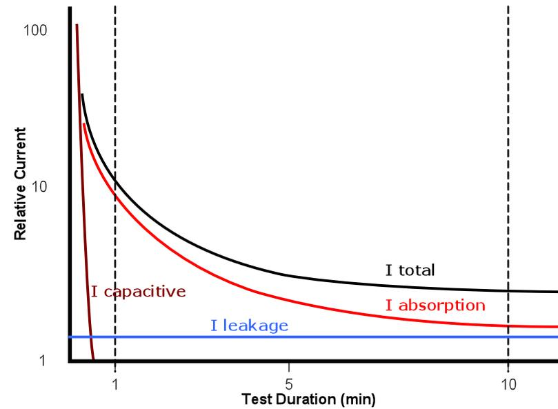
Measurements up to 100 GΩ can be made without any special precautions, assuming that the test leads are reasonably clean and dry. The guard lead can be used to remove the effects of surface leakage if necessary. When measuring resistances above 100 GΩ, the test leads should not be allowed to touch each other, or any other object since this will introduce leakage paths. Sharp points at the test lead connections should also be avoided since this will encourage corona discharge.
