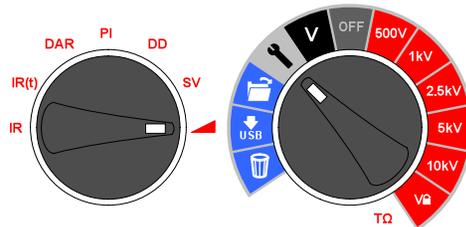
The test will ramp the voltage until it reaches the selected test voltage unless a breakdown or sudden rise in current is detected. The result displayed after the test is the final insulation resistance, voltage and current. If the result is saved a complete curve of current ( $\mu A$ ) and voltage (kV) is recorded and can be read into PowerDB, PowerDB Lite or converted to a spreadsheet so that the current vs. voltage curves can be compared to published curves in IEEE 95-2002.
