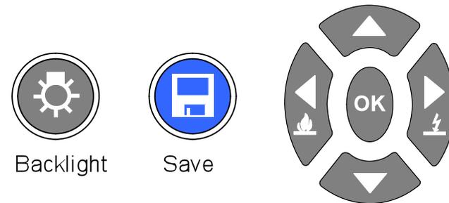
*Four arrow buttons and OK facilitate adjustment and selection of settings, voltages and modes. Breakdown/burn modes are set using the left and right arrow buttons. Backlight and save functions are dedicated buttons. All models have backlight and the MIT525 and MIT1025 have the Save button.*
