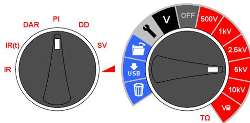
It is possible to adjust the test voltage using the up and down arrow buttons, either before or during a test. Once a test has begun, it is advisable to only adjust the voltage in the first 10s of the test to prevent interference with the capacitive and absorptive currents in the insulator.
