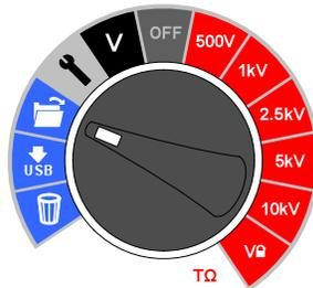
In saved results, the test mode is identified by the icon or abbreviation of each test on the display. In addition, the open folder icon is displayed to indicate recall memory mode.
