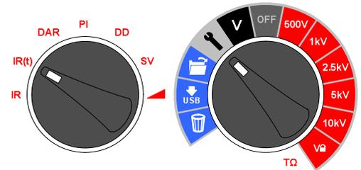
Turn the central rotary switch to the settings position. Select IR(t) on the test mode rotary switch. The default time of 1:00 minute will flash prompting the user to select a new time using the up/down arrow buttons. Press OK to set test duration and turn central rotary switch to desired test voltage. Press and hold TEST to start the test.
