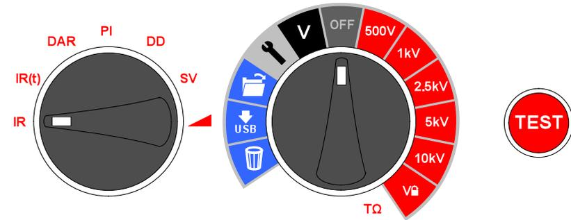
*Instrument controls are simple to operate. The central rotary switch incorporates the OFF position. The left hand rotary switch selects insulation test type (test mode switch). The TEST button starts and stops a test.*
