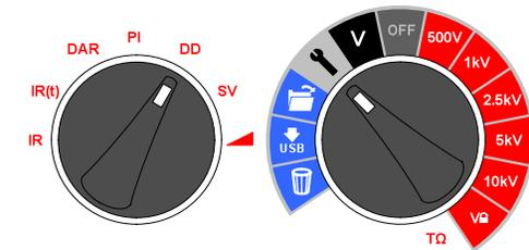
diagnostic insulation test that allows ageing, deterioration, and voids in the insulation to be assessed. The result is dependent on the discharge characteristic so the internal condition of the insulation is tested, largely independent of any surface contamination.
