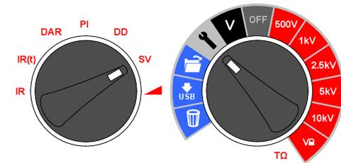
The step timer will always be set to total test time divided by five. Too short a step time may result in incorrect readings and too long a step time may over stress a motor.
