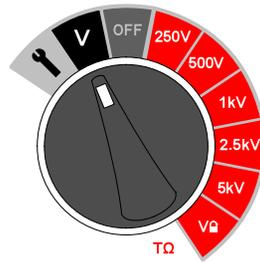
The voltmeter can be used to confirm that the insulation is discharged and for general purpose use. Positive and negative terminals are used for the voltmeter function; do **not** connect the GUARD terminal in **voltmeter mode**.
