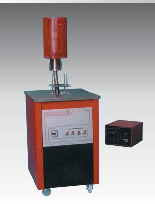
A disadvantage of many fluidized-bed baths is that good temperature stability and uniformity cannot be achieved in the fluidized medium itself. They are obtained by using large metal blocks or by inhibiting the fluidizing action in the powder around the work piece - either locally, or by completely collapsing the bed at the required temperature, this is not the case with the 875. A full evaluation report is available upon request.
