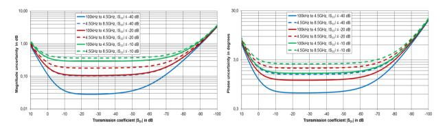
Typical accuracy of transmission magnitude and transmission phase measurements for the R&S $^{\circ}$ ZND Analysis conditions:  $S_{11} = 0$ , cal. power -10 dBm, meas. power -10 dBm, Base unit or R&S $^{\circ}$ ZND-K1 installed.
