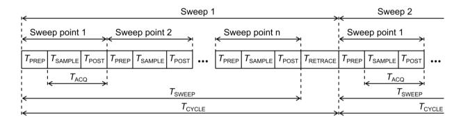
$T_{PREP}$  Preparation time required to set up the internal hardware components
