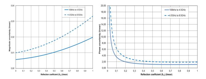
Typical accuracy of reflection magnitude and reflection phase measurements for the R&S®ZND Analysis conditions:  $S_{12} = S_{21} = 0$ , cal. power – 10 dBm, meas. power – 10 dBm, R&S®ZND-K5, R&S®ZND-K6 or R&S®ZND-K8 installed.
