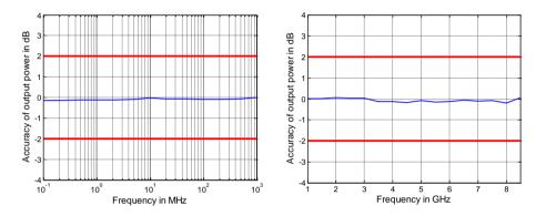
Output power accuracy in dB versus frequency for the R&S®ZND base unit.
