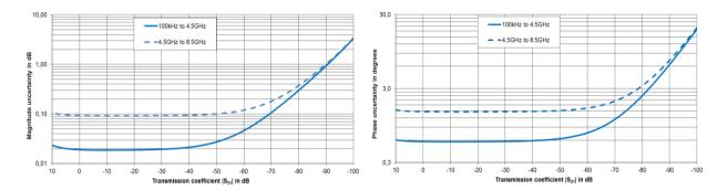
Typical accuracy of transmission magnitude and transmission phase measurements for the R&S $^{\circ}$ ZND Analysis conditions:  $S_{11} = S_{22} = 0$ , cal. power –10 dBm, meas. power –10 dBm, R&S $^{\circ}$ ZND-K5, R&S $^{\circ}$ ZND-K6 or R&S $^{\circ}$ ZND-K8 installed.
