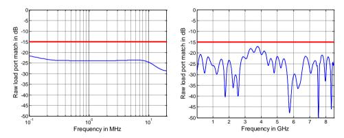
Raw load port match versus frequency for the R&S®ZND.
