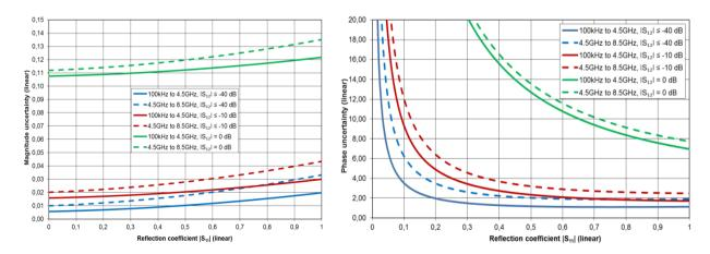
Typical accuracy of reflection magnitude and reflection phase measurements for the R&S $^{\circ}$ ZND Analysis conditions:  $S_{21} = 0$ , cal. power -10 dBm, meas. power -10 dBm, Base unit or K1 installed.
